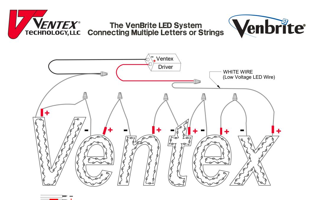
Positive wire to be taped with red tape (or equivalent marking) NOTE: Marked (Taped) wire ALWAYS ties to unmarked (non-taped) wire
